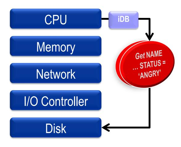
The communication between CPU and Disk carries the information on the query – columns and predicates. This occurs as a result of a special protocol called iDB.
